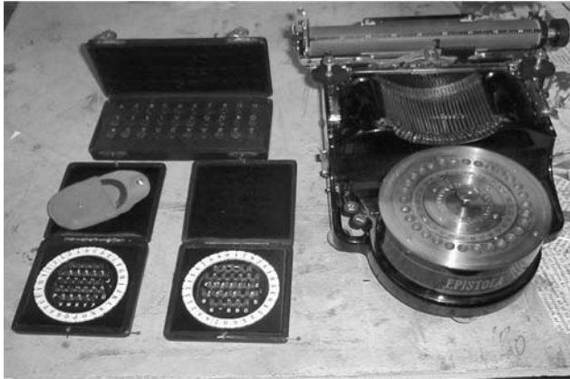
Figure 4. Cryptograph "EPISTOLA" (version IV) (1914–15).
