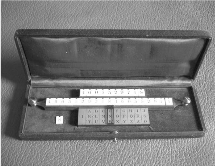
Figure 9. Cipher slide with ivory figures.
